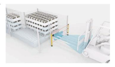
Solution: Access to the danger zone is safeguarded by a multiple light beam safety device. A sensor for detecting the forklift truck is installed behind this. By evaluating the sensor signals and their sequence, the safety system distinguishes between forklift trucks and persons. Automatic restart is possible.
